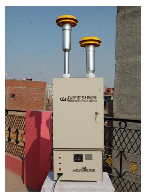
As per recent Air quality standard published by Govt. of India where measurement of PM 2.5 dusts has been made mandatory besides other parameters for defining the quality of ambient air. An impactor based PM 2.5 sampler has been manufactured by Lata Envirotech Services which is meet requirements of PM10 & PM 2.5 sampling using APM 250. PM 10 & PM 2.5 concentration in ambient air can be measured by using this sampler simultaneously.
